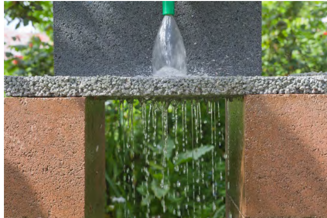
Porous concrete is another solution to excess stormwater run-off that preserves the look of traditional concrete
